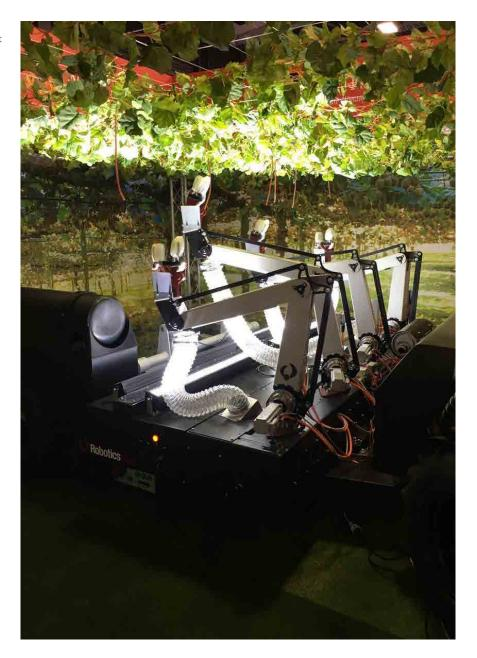
Right: Robotics Plus robotic kiwifruit harvesting autonomous vehicle
