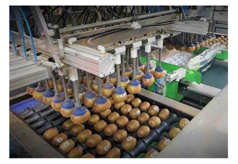
Initial testing on site in the 2019 kiwifruit season showed that the Pacmaster could consistently pack 22 trays of kiwifruit per minute. This is a significant change compared to older tray packing versions at 15 trays per minute or the 3 trays per minute achieved on average by packing staff per outlet on a sizer.
