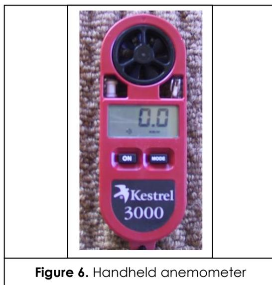
**Figure 6.** Handheld anemometer
