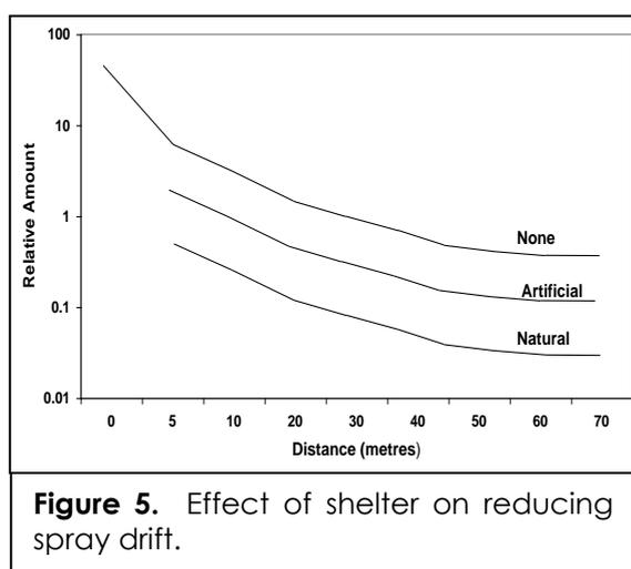
**Figure 5.** Effect of shelter on reducing spray drift.
