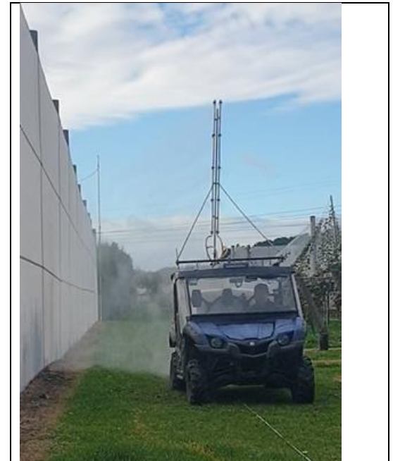
Figure 3: Testing drift reduction from artificial shelter in a 2 m/s wind. Approximately 50% of the droplets that reached the shelter passed right through this single layer artificial shelter.
